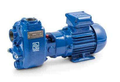
**Product Data** Suction port Threaded - 1"1/2 ISO 228 (BSP) Delivery port Threaded - 1"1/2 ISO 228 (BSP) Qmax 25 m<sup>3</sup>/h - 416 l/min (110 USgpm) Hmax 23 m (75 ft) Solids handling 20 mm (0.8") Motor power 2.2 kW - 3 HP Motor type **IEC** standard Winding for inverters **Cast iron frame** Motor brand WEG W22 Premium Weight 40 kg (88 lb)
